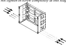
Step 5 Position the top panel in palce. Secure both sides of the panel using (3) M4 screws on each side. Now you can tighten all screws.
