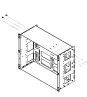
Step 6 (Optional) If center mount is required, you can install DP100 in between both 6U panel. This allows you to mount (1) Din Rail at center position.
