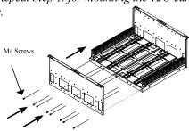
**Step 4** Take the Cover panel and place it with the flange facing up. Ensure that the short depth side cut is facing forward, as shown in the illustration. Attach the side brackets to the righ and left side of the cover panel using (3) M4 Screws for each bracket. However, do not tighten th screw completely at this stage.
